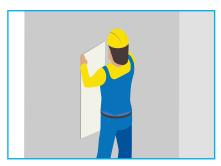
Position the mesh from the top to the bottom of the wall, pressing it into the base coat (starting from the center and moving outward).
