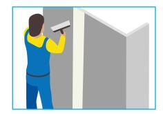
Apply the second layer of base coat, sandwiching the mesh between the two layers.
